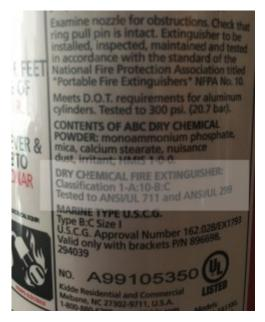
The rating for this fire extinguisher is 1A 10BC — as shown in the highlighted portion of the label.
