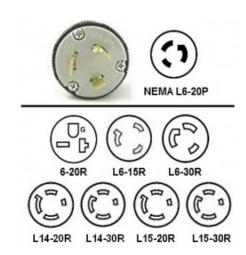
• Plug Types: 4 prong plugs can be 3 phase (3 hot / 1 ground), but all 3 prong plugs are single phase
